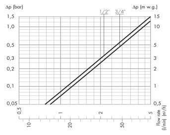
Recommended FLOW RATES to ensure stable operation and an accuracy of ± 2°C
